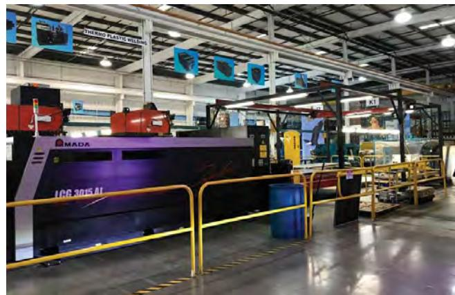
**CREATE:** At the Riviera Beach location, all fabrication is done in-house. Pictured here is a 4,000-W fiber laser with dual shuttle tables for high-speed metal cutting with material as thick as 7/8-inch steel plate.
