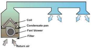
Return air from the house is filtered and blown through the air conditioner coil fins, which are chilled. The filtered return air is chilled by passing over, under and around the chilled aluminum fins and copper tubing.
