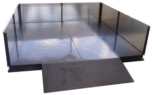
RGF's Portable Washpad requires no permits and can be operational in hours not weeks. Constructed of steel and aluminum with a 2 part epoxy coating for years of service, it has a built in washwater catchment trough with sump pump which sends the water to your recycling system for reuse or to discharge (if permitted). Two standard sizes are available and able to support large equipment Up to 20,000 lbs. Built in ramp makes access simple. Custom sizes are available.
