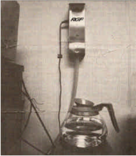
RGF Environmental's ice-maker sanitizer (above coffee pot) pumps gas into the machine (at left) to kill Listeria bacteria, which can live on ice
