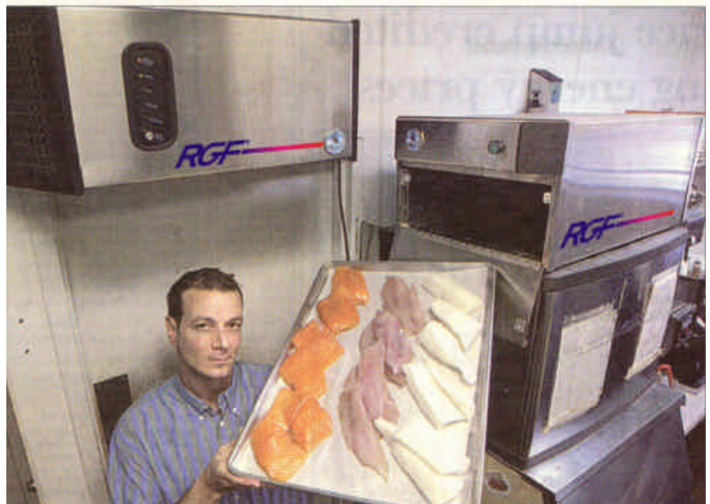
Food can be put in the bacteria-killing box to restauranteur Rick Orsi's left, while the unit above him cleans the air.
